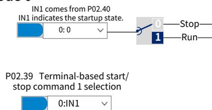
Only check IN1 (P02.40) input (0: Stop; 1: Run): when IN1 is 0, OFF1 is 0; when IN1 is 1, OFF1 is 1.
