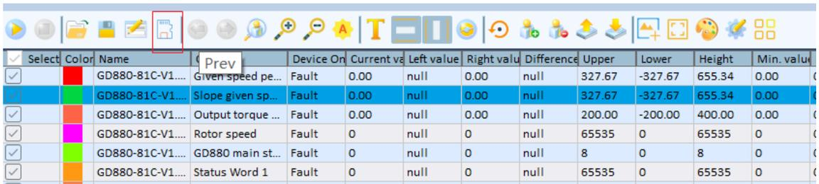
Step 3 In the window that is displayed, select the **WaveLog** folder where the fault waveform data is stored.
