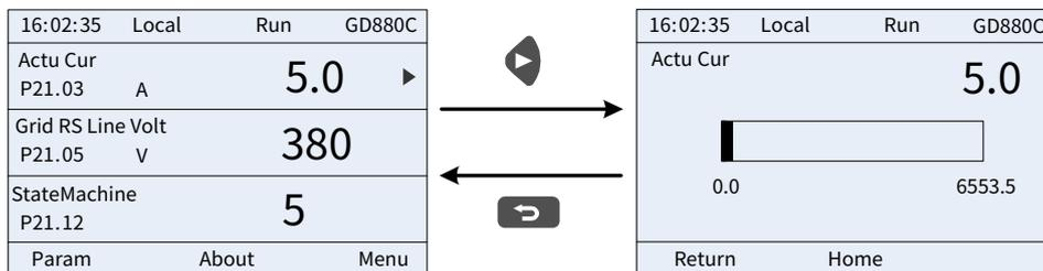
Under running state, multiple kinds of state parameters can be displayed. The running display parameter list is user defined, and each state variable function code can be added to the running display parameter list as needed. The state variable which has been added to the running display parameter list can also be deleted or shifted.
