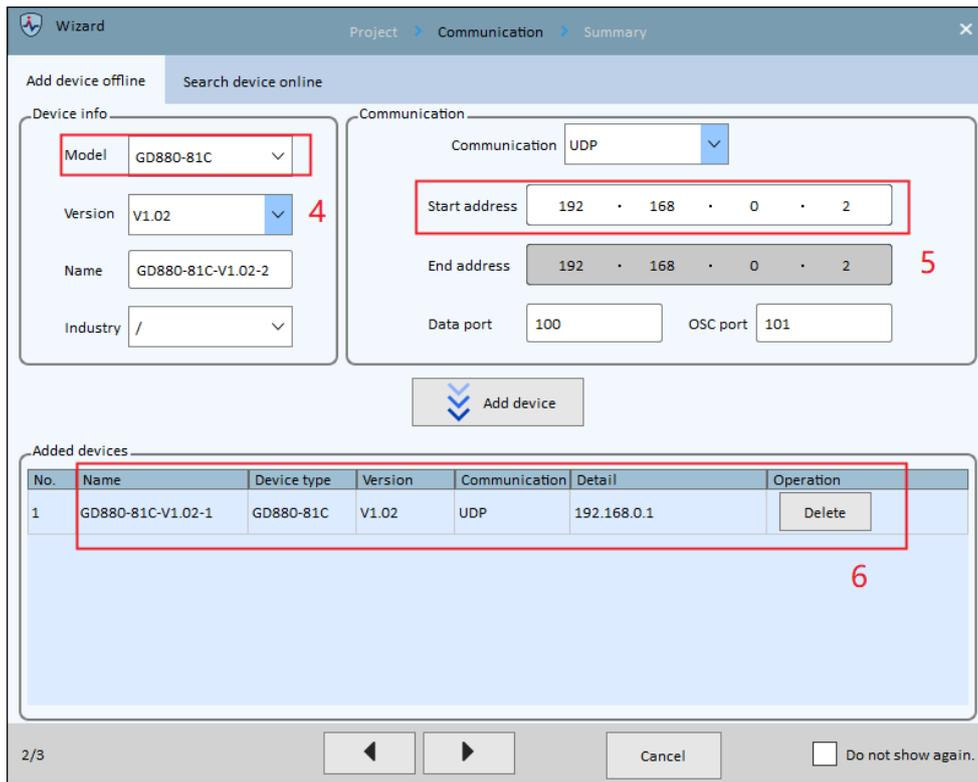
Step 7 Verify the device type, version, communication type, and communication details again.
