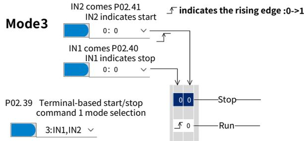
Check the inputs of IN1 (P02.40) and IN2 (P02.41): when IN2 is 0 and IN1 generates a rising edge, OFF1 is 1; when IN2 is 1, OFF1 is 0.
