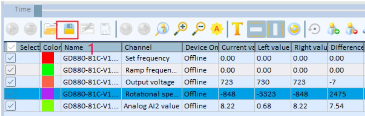
Step 2 The following window is displayed. If you also select **Export funcodes(.csv)** at the same time, all present function code values are automatically exported as a database file (CSV file). When saving waveforms, you can select the format of file to export and channel waveforms(all channel waveforms are exported by default).
