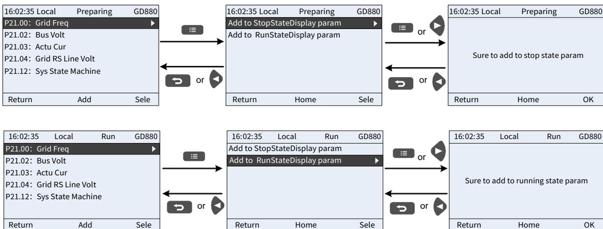
Press the key to enter the addition interface, select the operation needed, and press the key, key or key to confirm the addition operation. If the key or key is pressed without selecting the addition operation in "Add", it will return to the monitoring parameter list menu.
