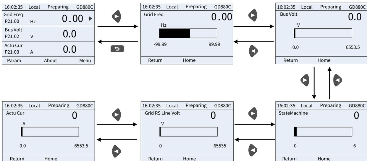
The stop display parameter list is user defined, and each state variable function code can be added to the stop display parameter list as needed. The state variable which has been added to the stop display parameter list can also be deleted or shifted.
