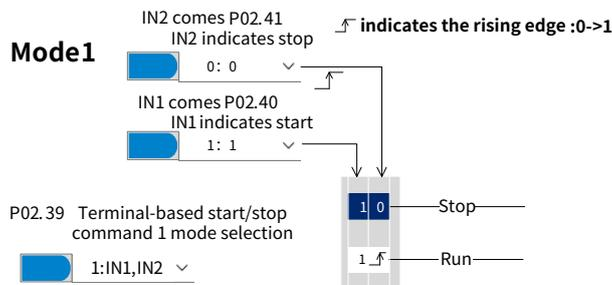
Check the inputs of IN1 (P02.40) and IN2 (P02.41): when IN1 is 1 and IN2 generates a rising edge change, OFF1 is 1; when IN1 is 0, OFF1 is 0.
