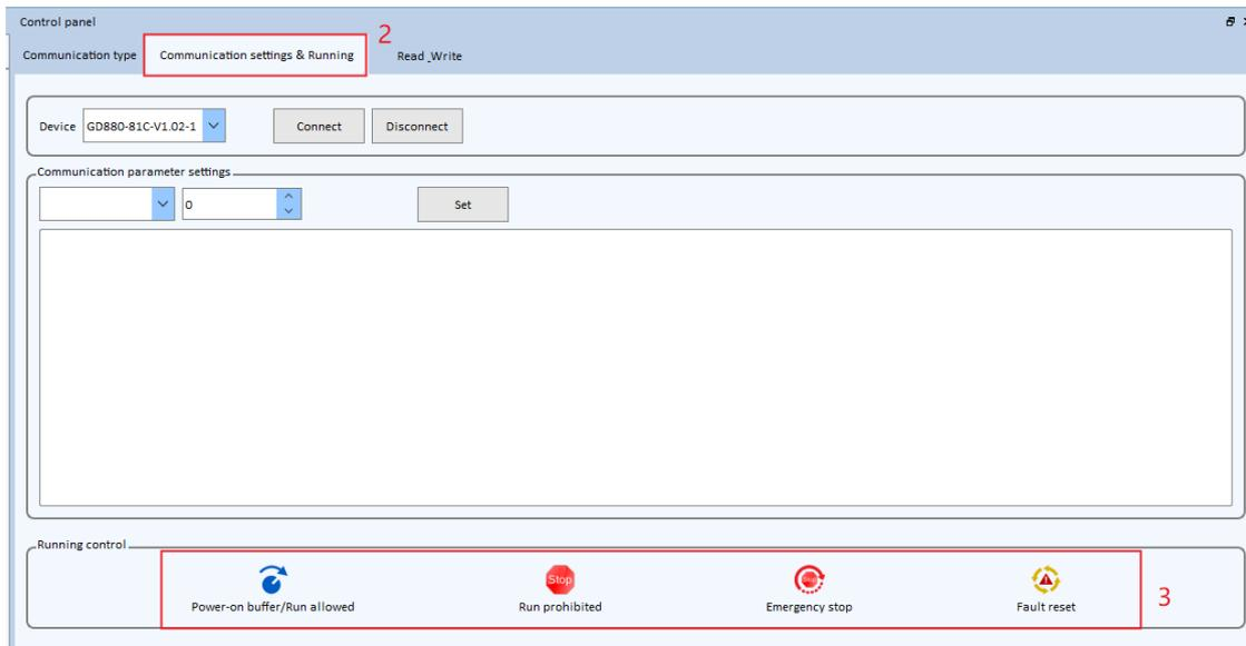
Step 3 The read/write testing supports the operation on any device, supports the connection to or disconnection from the device, and supports clearing result records.
