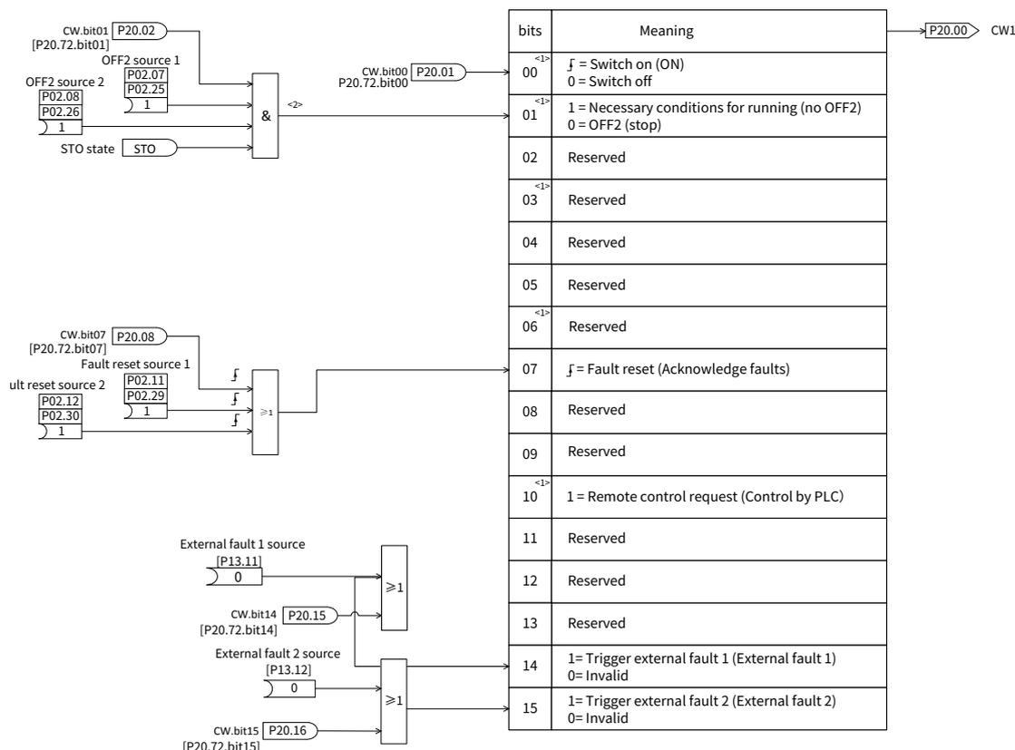
**Note:** If the PLC controls start/stop, bit 10 of CW 1 must be set to 1.
