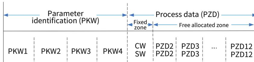
By using the 32 inputs/outputs, you can set the reference parameters of VFD, monitor the state values, transmit control commands, monitor the running state, and read/write the function parameters. For specific operations, see the following description.
