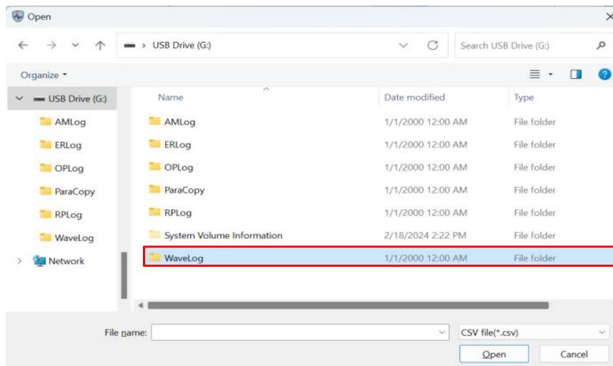
Step 4 Open the waveform data you want to view based on the recorded time. Select **Num\_02.csv** if you want to open the most recent fault waveform.
