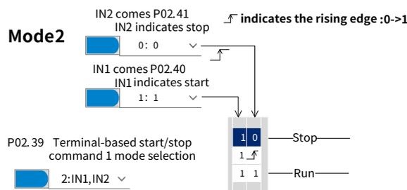
Check the inputs of IN1 (P02.40) and IN2 (P02.41): when IN1 is 1 and IN2 generates a rising edge and remains high level, OFF1 is 1; when IN1 is 0 or IN2 is 0, OFF1 is 0.
