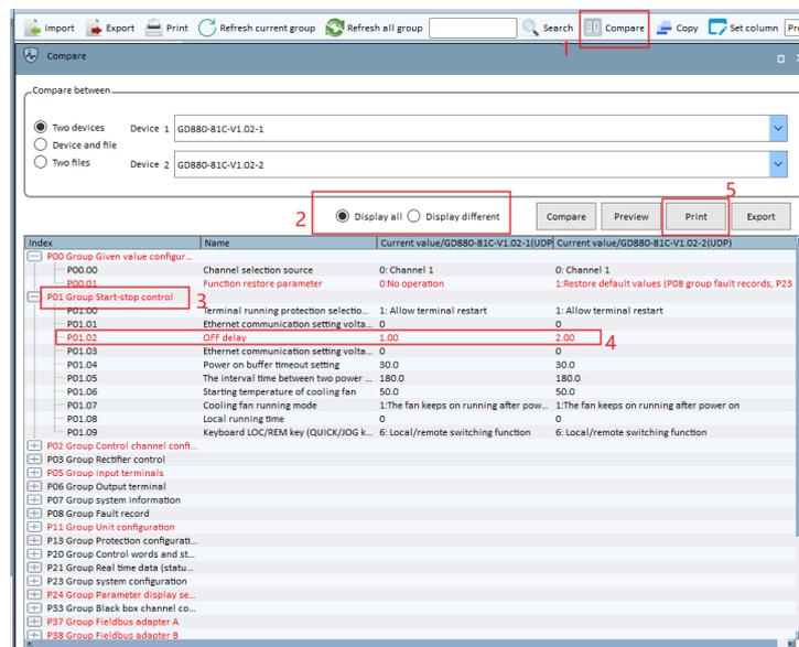
5. Printing comparison function codes allows you to print all values or different values. The following is a print preview interface example for all values. The format is the same as that of the current comparison function code interface.
