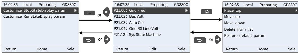
Press the key to enter the edit interface, select the operation needed, and press the key, key or key to confirm the edit operation and return to the previous menu (parameter list). The returned list is the list edited. If the key or key is pressed in the edit interface without selecting the edit operation, it will return to the previous menu (while the parameter list remains unchanged).
