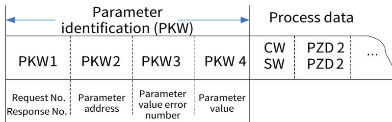
In the process of periodic communication, PKW zone is composed of four words (16 bit), each word is defined as follows:
