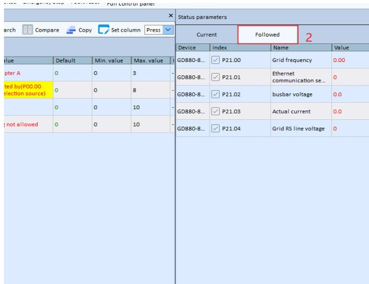
Step 3 The status window can be hidden or closed. When hidden, the status window is displayed vertically; when closed, the status window will not be displayed, but the status parameters can be redisplayed by choosing **View > State parameters**.
