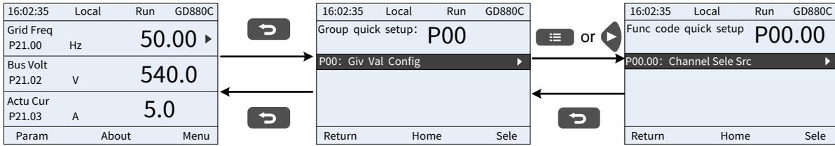
The following figure shows how to enter or exit different level menu step by step, as shown in the following figure.
