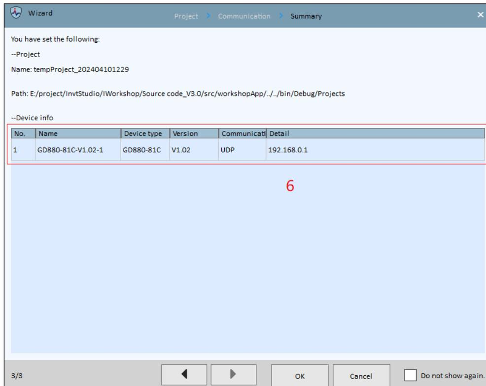
Step 7 Verify the device type, version, communication type, and communication details again.
