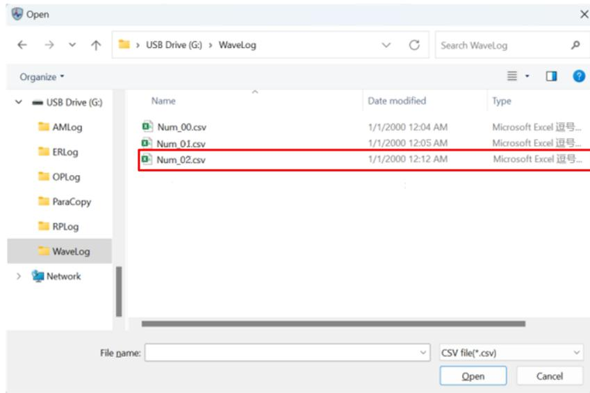
Step 5 The open waveform is the SD card fault waveform saved at the fault time, and the fault waveform data matches the channel configured in group P33.
