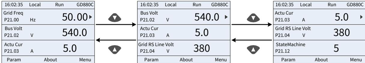
Press or to switch between different display styles, including list display and progress bar display.
